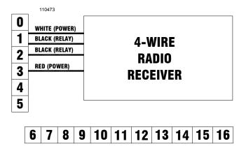
Figure 16: Wiring 4-Wire Receiver
